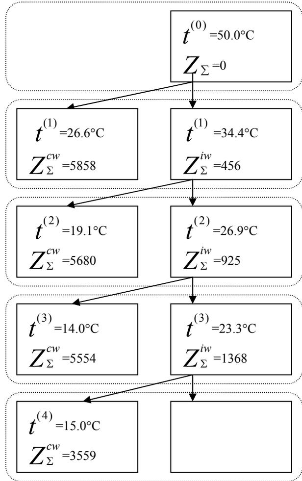
Fig. 4. Tree of possible thermoecconomical expenditure the system of chlorine water refrigeration
