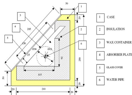
Fig. 9. Schematic of the experimental apparatus cross section
