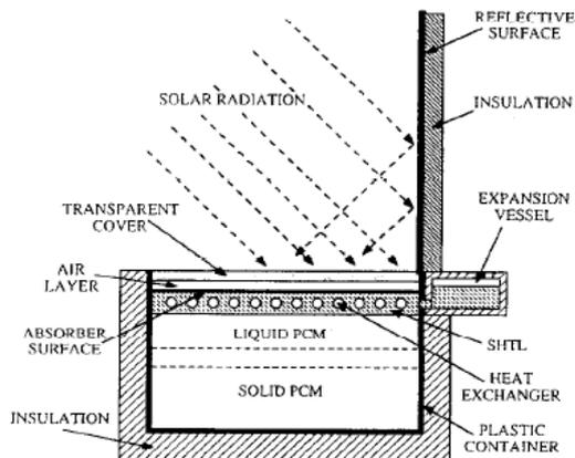
Fig. 4. Schematic presentation of the integrated solar collector storage system based on a phase-change material
