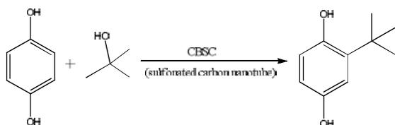
Scheme 7. Catalytic alkylation of hydroquinone with tert-butanol
