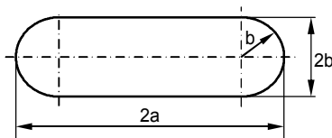
Fig. 1. The geometrical parameters of square duct with rounded corners
