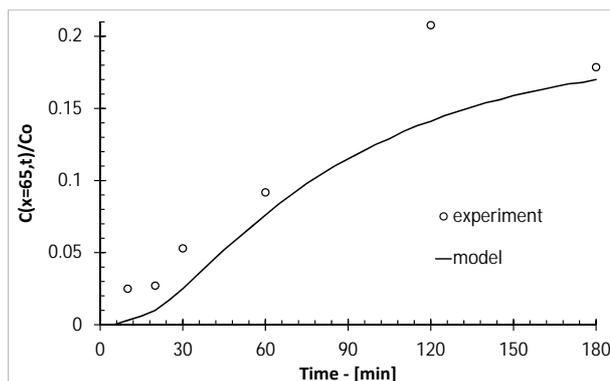
Fig. 5. Tracer concentration behavior for sampling position  $x = 60\text{cm}$
