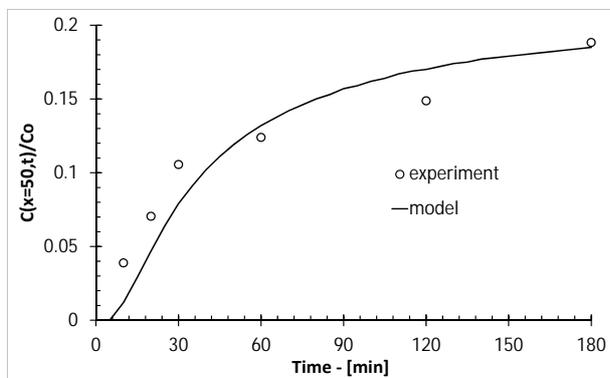
Fig. 4. Tracer concentration behavior for sampling position  $x = 50\text{cm}$
