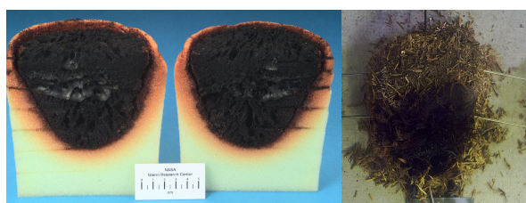
Fig. 2. Left) Cross-section of a partly smouldered polyurethane slab 200 mm high burned in microgravity conditions (photo by NASA, [12]). Right) Smouldering of a 80 by 50 mm sample of woody fiberboard (31 min after hot-coil ignition at the bottom)
