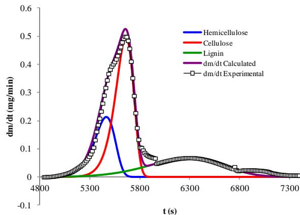
Fig. 4. Adjustment by deconvolution of the three components of rice husk
