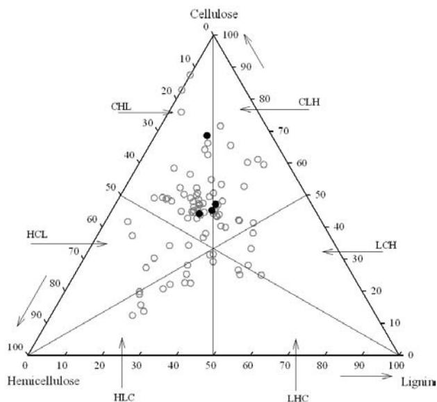
Fig. 5. Ternary composition diagram of hemicellulose, cellulose and lignin of different biomass
