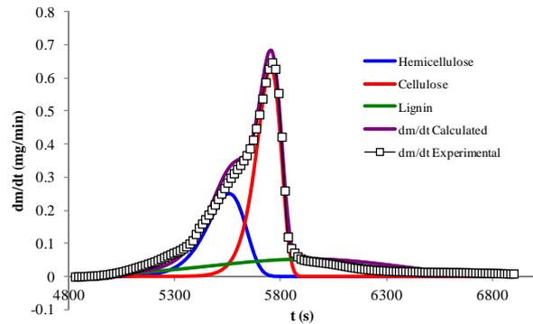
Fig. 3. Adjustment by deconvolution of the three components of pine sawdust
