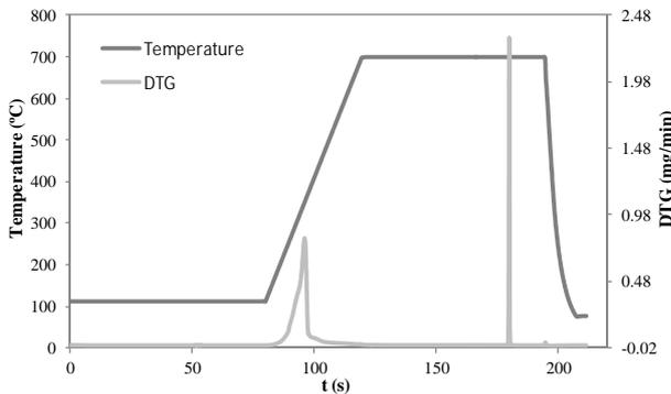
Fig. 1. DTG curve obtained in the test performed at ramp 15 °C/minute
